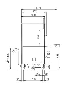
Drain ΕI Electrical inlet (power) EO **Electrical Outlet** HWI Hot water inlet ΧD Detergent connection XR = Rinse aid connection
